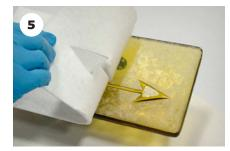
Be sure to wear respiratory protection as you peel away the fiber paper. Remove any residue with a scrub pad or nylon brush and water.
